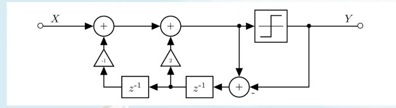
provides further shaping of the quantization noise:  $Y = X + Q(1 - z^{-1})^2$
