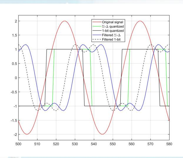
no advantage to  $\Sigma\Delta$  here despite oversampling, over-driven ADC
